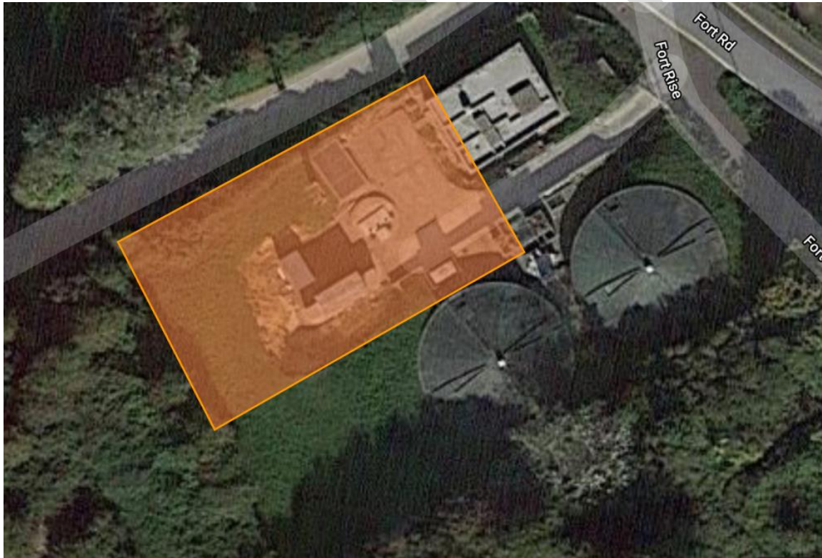
Figure 23- The footprint of a 35x20m EfW plant is marked out alongside the sewage treatment works. This would benefit from the EfW plant's electrical supply and already has a grid connection in place for backup. The generators could be decommissioned.
