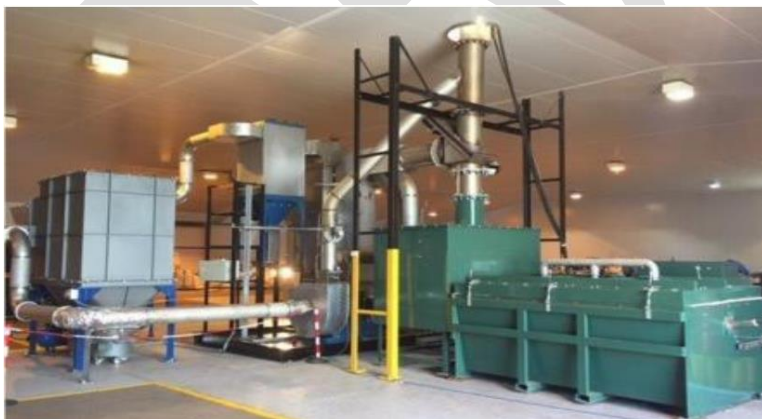
Figure 27- A modular EfW plant
